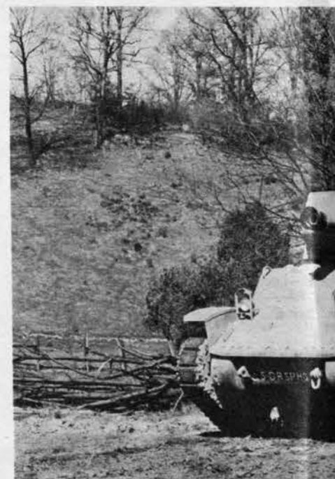
U. S. M-8, a self-propelled 75-mm. howitzer, has a chassis and suspension resembling that of M-5A1 shown at top. A
